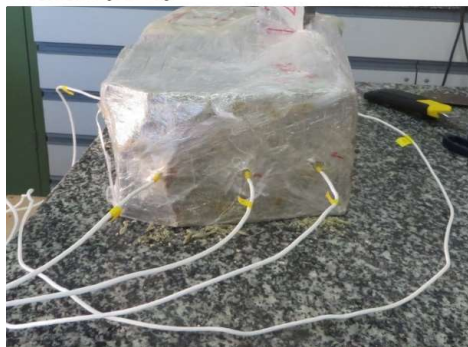
Measurement of suction in the lab with psychrometers
