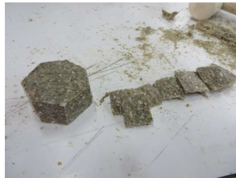
Splitting the core in two, removing external parts, smoothing surfaces
