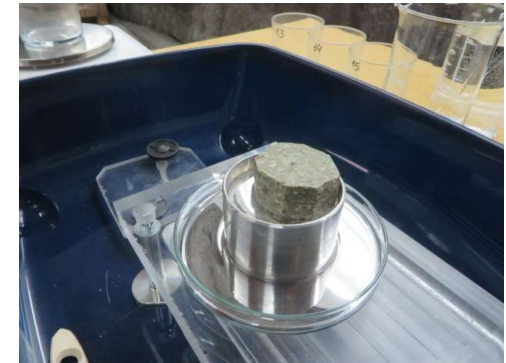
Immersion of the samples in mercury to determine its volume before drying in the oven
